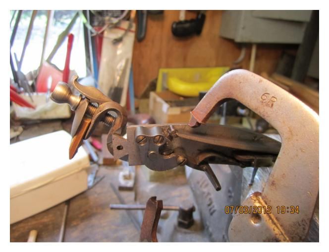
End of Removing the Main Spring
